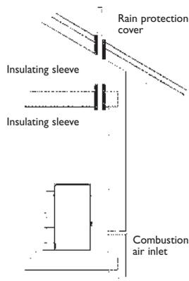
If the stove is to be installed in an existing chimney flue built into the wall, the pipe should be installed along the whole length of the chimney flue in order to prevent condensation that would mark the walls.
