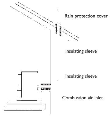
If the gas exhaust pipe is installed as in the drawing on the right, a rain protection cover will be needed in addition to the requirements listed above.
