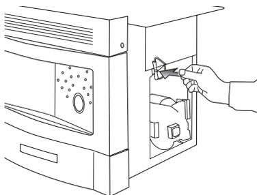
*Note that the thermal switch can only be reset with electrical supply off and when the stove temperature has fallen below 93°C.*
